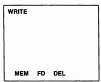
Press the  $\overbrace{F2}$  (FD) key to show the setup screen for the file name used when copying data to a floppy disk.
