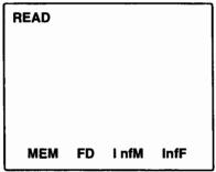
To view information on the internal memory, press the  $\stackrel{\frown}{\vdash}_3$  (InfM) key; to view information on the floppy disk, press the  $\stackrel{\frown}{\vdash}_4$  (InfF) key. In this example, press the  $\stackrel{\frown}{\vdash}_4$  key to open the screen for choosing a file.
