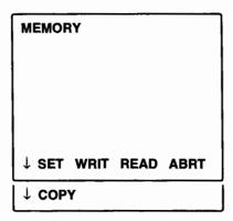
Press the  $\bigcap_{MEMORY}$  function key to open the menu screen. Press the  $\bigcap_{F2}$  (WRIT) key to open the WRITE setup screen.
