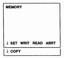
Press the  $\overbrace{\text{MEMORY}}$  function key to open the menu screen. Press the  $\overbrace{\text{NEXT}}$  key and then the  $\overbrace{\text{F1}}$  (COPY) key to open the COPY menu screen.
