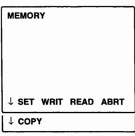
Press the  $\bigcap_{MEMORY}$  function key to open the menu screen. Press the  $\bigcap_{F3}$  (READ) key to open the READ
