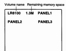
The screen shows the volume name and the amount of free space on the floppy disk as well as the names of the setup data files saved on the floppy disk. Using the  $\Delta/\nabla$  keys, choose the setup data file you want to delete. Pressing the ENTRY key deletes the selected file.
