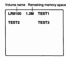
The screen shows the volume name and the amount of free space on the floppy disk as well as the names of the data files saved on the floppy disk. Using the  $\triangle / \nabla$  keys, choose the file for which you want the information shown. Pressing the ENTRY key shows the information on the selected file.
