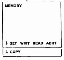
Press the  $\overbrace{\text{F3}}^{\text{MEMORY}}$  function key to open the menu screen. Press the  $\overbrace{\text{F3}}^{\text{READ}}$  (READ) key to open the READ setup screen.
