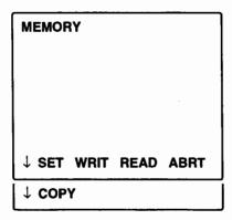
Press the MEMORY function key to open the menu screen. Press the  $F_3$  (READ) key to open the READ menu screen
