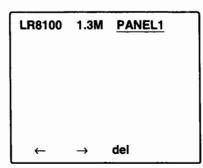
The screen shows the volume name and the amount of free space on the floppy disk. With the alphanumeric keypad and the  $\overbrace{F1}$ ,  $\overbrace{F2}$  and  $\overbrace{F3}$  keys, type in the file name using no more than eight characters. Pressing the  $\boxed{\text{ENTRY}}$  key saves the setup data.
