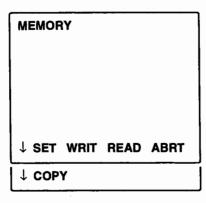
Press the  $\overbrace{\text{MEMORY}}$  function key to open the menu screen. Press the  $\overbrace{\text{F1}}$  (SET) key to open the SET setup
