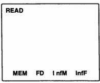
Press the  $\bigcap_{F_1}$  (MEM) key to open the setup screen for reading conditions.
