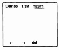
The setup screen then shows the volume name and the amount of free space on the floppy disk. With the alphanumeric keypad and the  $F_1$   $F_2$  and  $F_3$  keys, type in the file name using no more than eight characters. Pressing the ENTRY key shows the setup screen for writing conditions.
