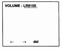
With the alphanumeric keypad and the  $\bigcap_{F1}$ ,  $\bigcap_{F2}$  and  $\bigcap_{F3}$  keys, type in the volume name using no more than six characters. Pressing the ENTRY key formats the floppy disk.
