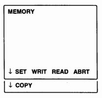
Press the MEMORY function key to open the menu screen. To delete a setup data file, press the SET) key to show the SET menu screen. To delete a measurement-data file, press the E2 (WRIT) key to show the WRITE menu screen.
